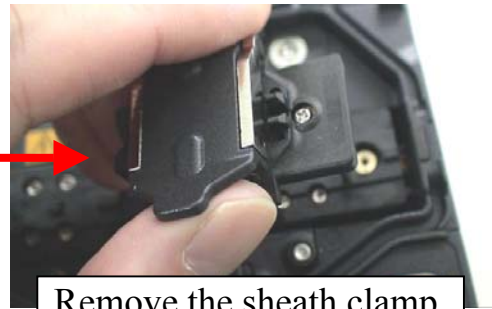
Remove the sheath clamp
